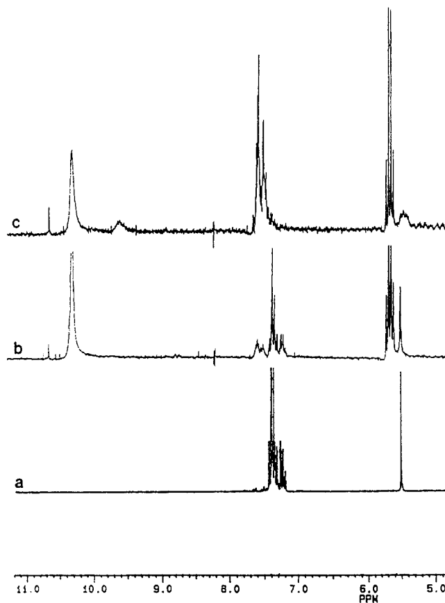
Figure 6. 200-MHz 1 H NMR spectra in DMSO- d 6 of (a) thiophenol, (b) trifluoroalanine NCA and thiophenol a few minutes after the preparation of the sample, and (c) the same sample after 18 h.
